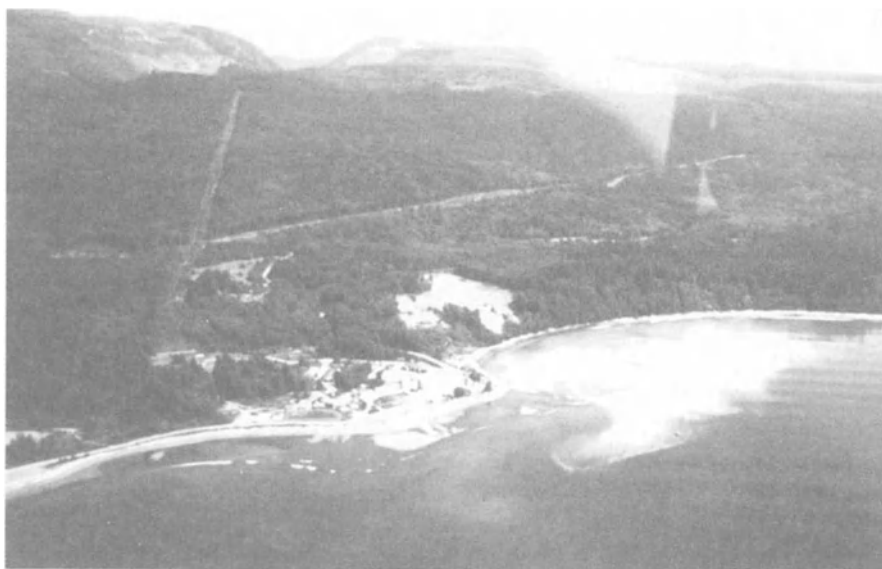
Fig. 9.3. At Jordan River Mine, the tailings line broke repeatedly and discharged tailings along shore. The oceanographic conditions and the pipeline design causing this are now known and can be avoided elsewhere
