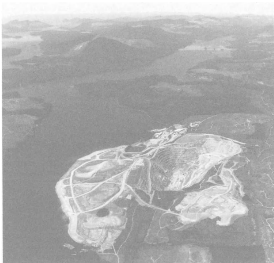
Fig. 9.4. At the Island Copper Mine, tailings were discharged for 25 years deep into adjacent fjord, where they deposited in the targeted area, with little surface turbidity. The pit is shown here, surrounded by waste rock under reclamation. The waste rock placed on the fjord side of the pit was to allow extension of mining right to the edge of the fjord. Subsequently, shallow embayments were cut into the dump edge to act as nursery areas for young salmon on their seaward migration from neighboring spawning streams. (From Island Copper Mine)
